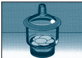
Cooling in a desiccator provides moisture-free, stable filter weights.
