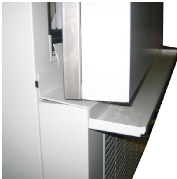
Figure 11: Unit door in drain off position above the drain well
