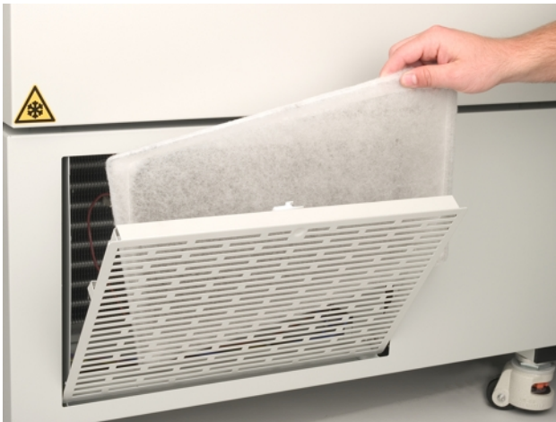
Figure 65: Taking out the filter
