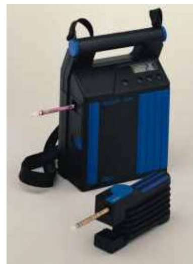
Example for hand pump (foreground) or a electrical pump (background)
