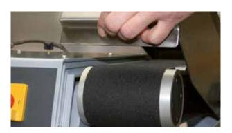
The Qgrind 100 is a stable wet double-belt grinder for deburring and pre-grinding of samples or other materials.
